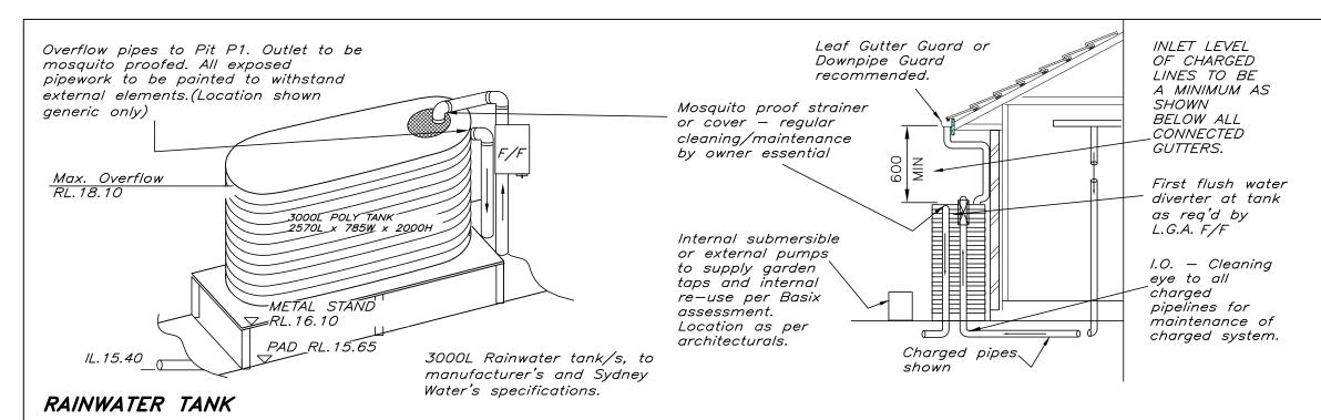
TANK DETAILS SHOWN ARE A SUGGESTED CONFIGURATION ONLY. ANY MODIFICATIONS TO TANK VOLUME OR INLET AND OUTLET LEVELS MUST BE APPROVED BY ENGINEER PRIOR TO COMMENCEMENT OF CONSTRUCTION. TANK SHAPE, & DEVICES SHOWN ARE DIAGRAMMATIC ONLY. MINIMUM OF 450 CLEARANCE (UNLESS L.G.A. REQUIRES LARGER SETBACK) TO SIDE BOUNDARIES MUST BE MAINTAINED. CLIENT IS RESPONSIBLE TO ENSURE COMPLIANCE WITH THIS IN THE INSTALLED STATE. Charged stormwater lines from Roof Areas ONLY to rainwater tank.
